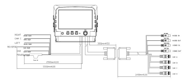
Screen size:7 Inch Panel (diagonal) Active area:154.08(H) x 85.92(V) Pixel configuration: 0.0642 x 0.179 Resolution:800(RGB) (W) x 480 (H)
